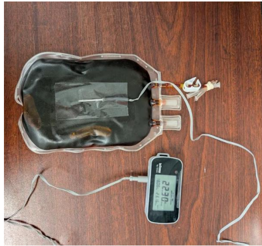
Figure 1. Temperature probe taped outside a payload simulant bag.
