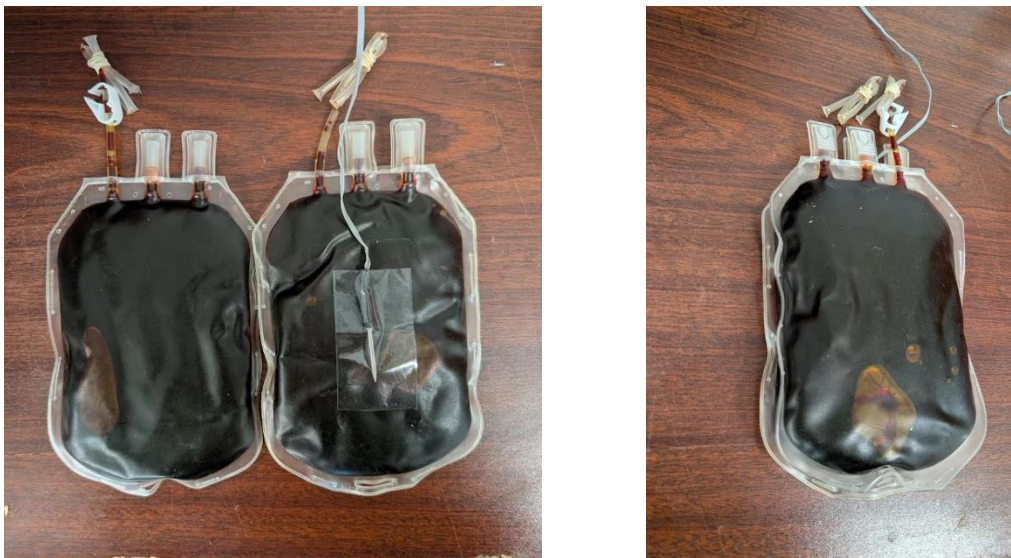
Figure 2. Temperature Probe sandwiched between two simulant units.
