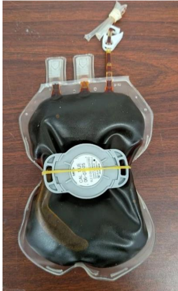
Figure 3. MaxConnect sensor affixed outside a payload simulant bag with rubber band.
